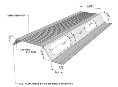
The resilient channel is used to provide a  $\frac{1}{2}$ " thick air barrier between two partitions, in order to reduce noise. The holes and the shorter side of the left leg allow air to circulate over the entire inner surface of the partition. It is usually used inside the building.
